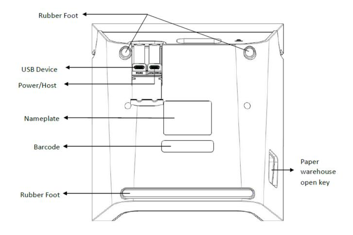
The matching diagram for A3700 host and B3700 printer base is as follows:
