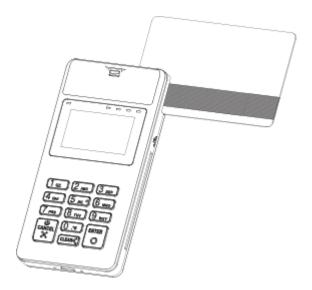
When swiping, the backside of the card must be faced up as shown in the image. Bidirectional swiping is supported.
