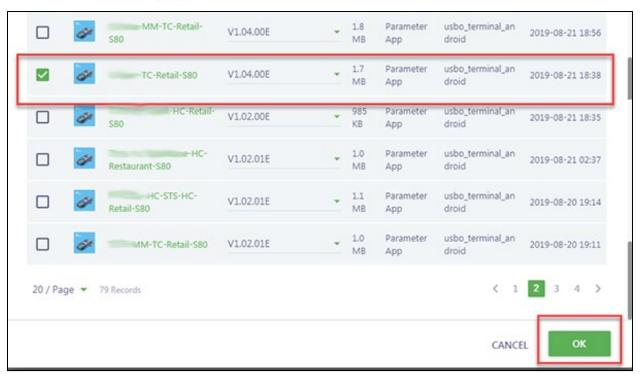
After selecting OK the parameter file page will display. It is required to complete the parameter file before pushing the application.
