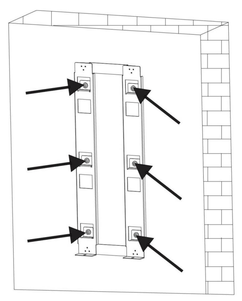
2. Use the four hooks on the back of the device to hang the device on the wall mount bracket. The hole diameter is  $8 \text{mm}\,.$
