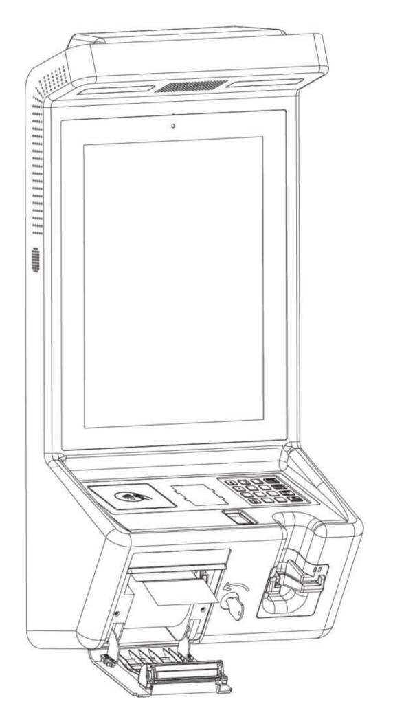
4. Close the printer cover and pull out the key. The printer will automatically cut off the extra paper.
