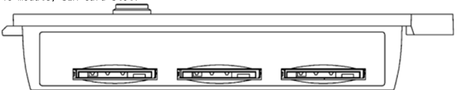
4G module, SIM (left) and SAM (middle and right) card slots.
