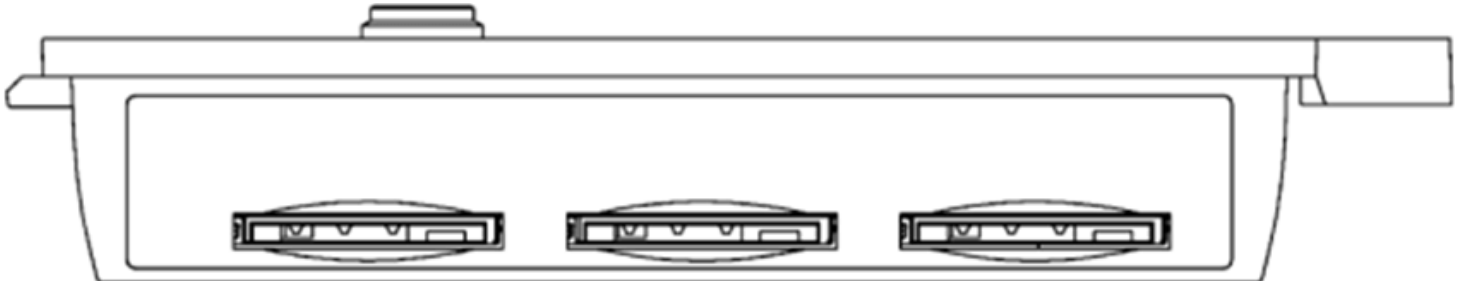
4G module, SIM (left) and SAM (middle and right) card slots.
