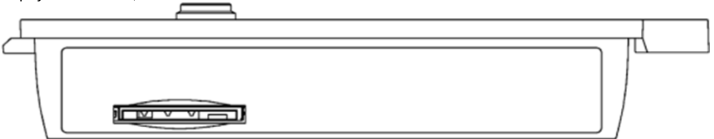
4G module, SIM card slot.
