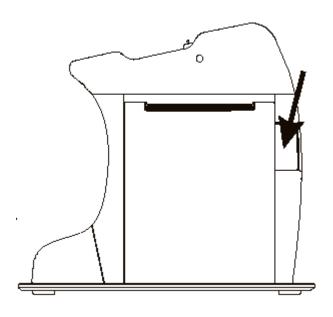
2. Load the paper roll into the paper compartment and extend the end of the paper out of the printer.
